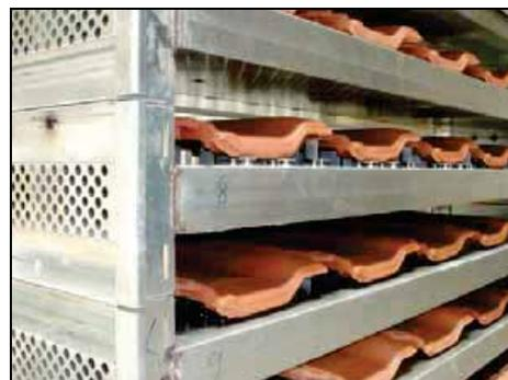
Figure 7: MobilSystem by Rotho- System of channel setters for roofing tiles <sup>49</sup>
